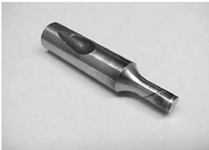
• Excessive heat due to tight clearance
